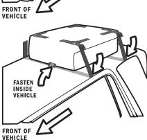
**C.** No Bars Rotate the 2 inch straps toward the sides of your vehicle. Open the doors and thread the straps through the interior of the vehicle and fasten together. Tighten the straps until they fit snugly; don't cinch so tight that you damage your roof.
